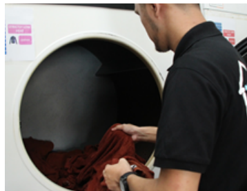
GAS FIRED DRYER - GIRBAU (SPAIN) 10 X 28KG MACHINES 9,000 KG/DAY
