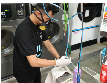
SPOTTING TABLE (TO REMOVE STAINS) - PONY (ITALY) 2 X MACHINES 200 PIECES/DAY
