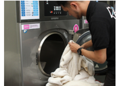
WASHER WITH WET CLEANING FUNCTION - GIRBAU (SPAIN) 6 X 23KG MACHINES 6 X 28KG MACHINES 9,000 KG/DAY
